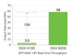
Projected performance subject to change, Token-to-token latency (TTL) = 50ms real time, first token latency (FTL) = 5,000ms, input sequence length = 32,768, output sequence length = 1,028, 8x eight-way DGX H100 GPUs air-cooled vs. 1x eight-way DGX B200 air-cooled, per GPU performance comparison.
